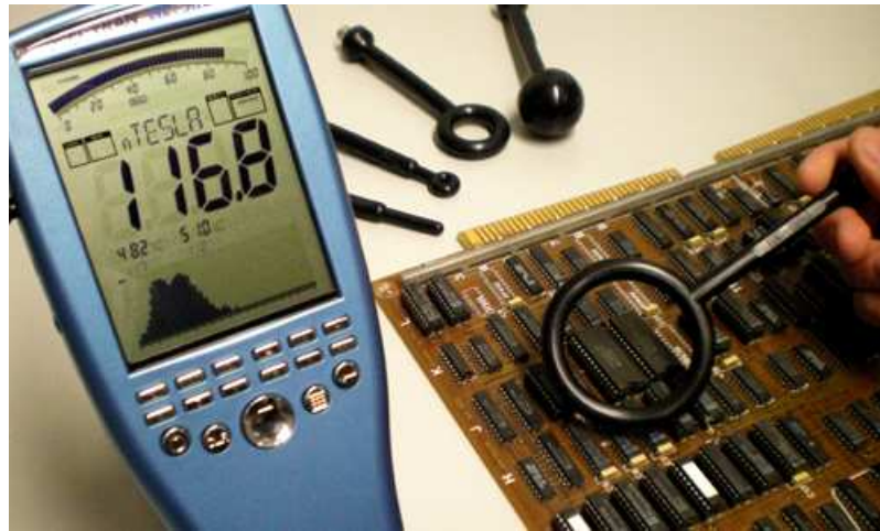
Magnetic field measurement on a group of components using the 60mm H-field probe
